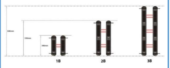
The **Dual Detection Technology** works by having a pair of Detectors (set 60 mm apart from each other) on each Beam, both Detectors have to be breached simultaneously to create an activation, allowing small animals, insects, leaves & debris to safely pass by.
